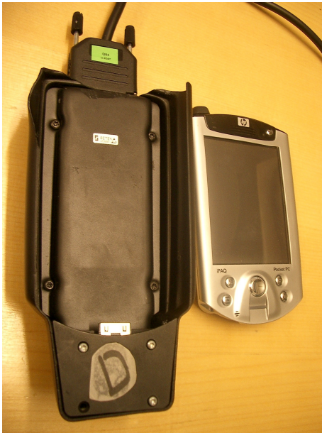
Figure 6 – The J1587 interface jacket and the TCU
